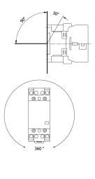
Dimensioned drawing installation contactors HS 3-024AC/63-22
