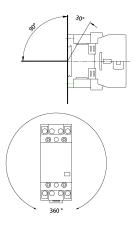
Dimensioned drawing installation contactors HS 3-024AC/63-40
