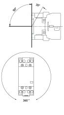
Dimensioned drawing installation contactors HS 1-230AC/20-20
