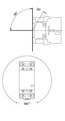
Dimensioned drawing installation contactors HS 1-024AC/20-20
