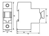
Dimensioned drawing fuse-switch-disconnector Tytan II Do-63-1/E
