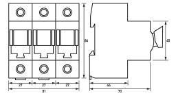
Dimensioned drawing fuse-switch-disconnector Tytan II Do-63-3/E  $\,$
