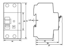
$Dimensioned\ drawing\ residual\ current\ operated\ circuit-breakers\ with\ integral\ overcurrent\ protection\ DRCBO\ 4\ C25/o, 30/1N-HP$
