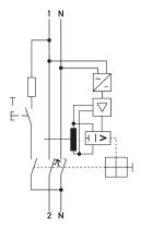
$Wiring example \ residual \ current \ operated \ circuit-breakers \ with \ integral \ overcurrent \ protection \ DRCBO \ 4 \ C25/o,30/1N-HP$
