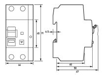
$Dimensioned\ drawing\ residual\ current\ operated\ circuit-breakers\ with\ integral\ overcurrent\ protection\ DRCBO\ 4\ C_{32}/o,30/1N-PV$
