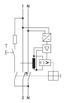
$Wiring example \ residual \ current \ operated \ circuit-breakers \ with \ integral \ overcurrent \ protection \ DRCBO \ 4 \ C_{32}/o, 30/1N-PV$
