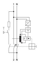
$Wiring \ example \ residual \ current \ operated \ circuit-breakers \ with \ integral \ overcurrent \ protection \ DRCBO \ 4 \ B25/o, 30/1N-B \ NK$
