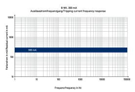
Diagrams residual current operated circuit-breakers with integral overcurrent protection DRCBO 4 B25/0,30/1N-B NK
