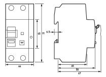
Dimensioned drawing residual current operated circuit-breakers with integral overcurrent protection DRCBO 4 B25/0,30/1N-B NK
