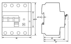
Dimensioned drawing residual current operated circuit-breakers with integral overcurrent protection DRCBO 4 C16/o,10/3N-HP
