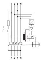
$Wiring example \ residual \ current \ operated \ circuit-breakers \ with \ integral \ overcurrent \ protection \ DRCBO \ 4 \ C16/o, 10/3 N-HP$
