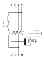
Wiring example residual current operated circuit-breakers with integral overcurrent protection DRCBO 4 C10/o,03/3N-A
