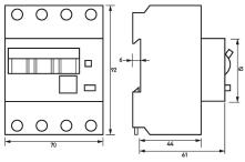
$Dimensioned\ drawing\ residual\ current\ operated\ circuit-breakers\ with\ integral\ overcurrent\ protection\ DRCBO\ 4\ C10/o,o3/3N-A$
