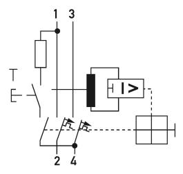
$Wiring example \ residual \ current \ operated \ circuit-breakers \ with \ integral \ overcurrent \ protection \ DRCBO \ 2 \ C_32/o, 30/2-A$
