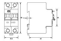
Dimensioned drawing residual current operated circuit-breakers with integral overcurrent protection DRCBO 2 C32/0,30/2-A
