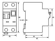
Dimensioned drawing residual current operated circuit-breakers with integral overcurrent protection DRCBO 3 Bo6/o,o3/1N-A
