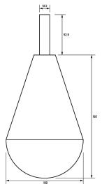
Dimensioned drawing float switches Champ 2 G-L/F HD 20 m  $\,$
