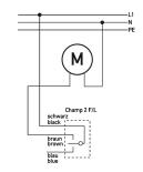
Wiring example float switches Champ 2 G-L/F 20 m
