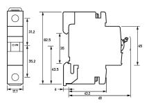
Dimensioned drawing miniature circuit-breakers DLS 6i Zo6-1
