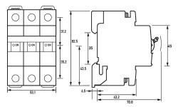
Dimensioned drawing miniature circuit-breakers DLS 6i K<sub>3</sub>,5-3
