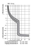
Diagrams miniature circuit-breakers DLS 6i K<sub>3</sub>,5-3
