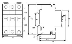
Dimensioned drawing miniature circuit-breakers DLS 6i B63-3
