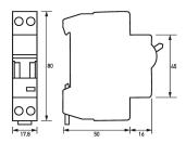
Dimensioned drawing miniature circuit-breakers ELS 3 B4o/1+N
