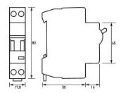
Dimensioned drawing miniature circuit-breakers ELS 3 B20/1+N
