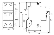
Dimensioned drawing miniature circuit-breakers DLS 6h B10-2
