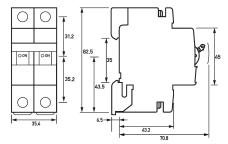
Dimensioned drawing miniature circuit-breakers DLS 6h B<sub>32-1+</sub>N
