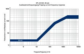
Diagrams circuit-breakers with residual current trip DFL 8 160-4/0,03-B SK
