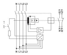
Wiring example circuit-breakers with residual current trip DFL 8 160-4/0,03-B SK
