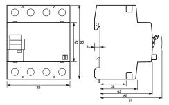
Dimensioned drawing residual current circuit-breaker DFS 4 063-4/0,10-HP
