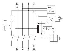
Wiring example residual current circuit-breaker DFS 4 063-4/0,10-HP
