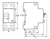
Dimensioned drawing residual current circuit-breaker DFS 2 040-2/0,30-HP HD
