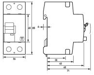
Dimensioned drawing residual current circuit-breaker DFS 2 025-2/0,10-HP
