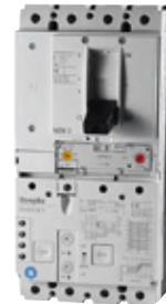
circuit-breakers with residual current protection are compact devices with an integrated auxiliary switch and terminals for large wire cross-sections of up to 185 mm<sup>2</sup>. They have a high short-circuit switching capacity and an adjustable response
