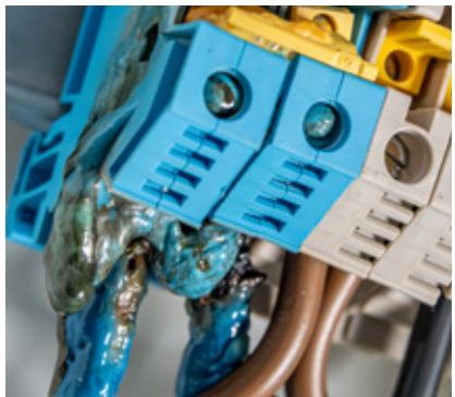
One of the most common causes of damage to electronic equipment is an interruption of the neutral conductor. If the line conductors are loaded asymmetrically, this results in a neutral point shift, which in turn causes overvoltage or undervoltage. The consequences may include damage or malfunction of connected electronic devices, or, in the worst case, fires.
