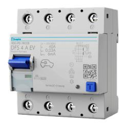
Another way to protect a charging station against residual currents is to combine a monitoring module for 6 mA DC detection with an additional Type A or Type F RCD. When working with this particular combination, the person or company responsible for the installation must, however, always carefully follow the switch-off criteria required in the event of a fault and be able to demonstrate that they have done so in cases of doubt.
